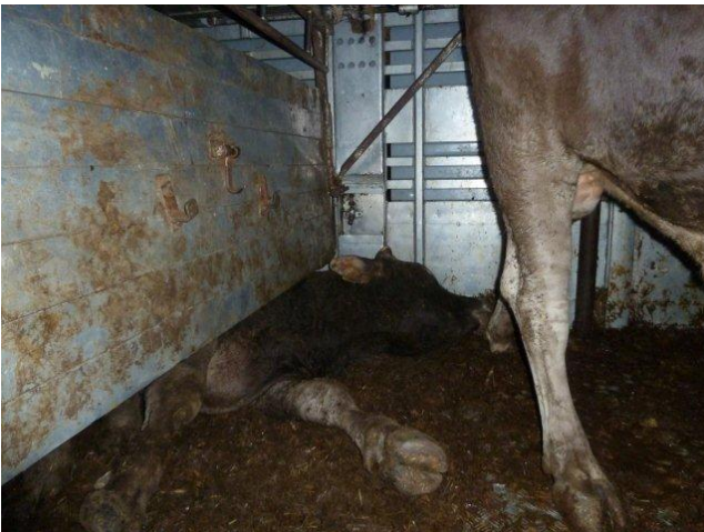
Gap between bottom of partition & floor – can result in legs getting stuck & injured.
