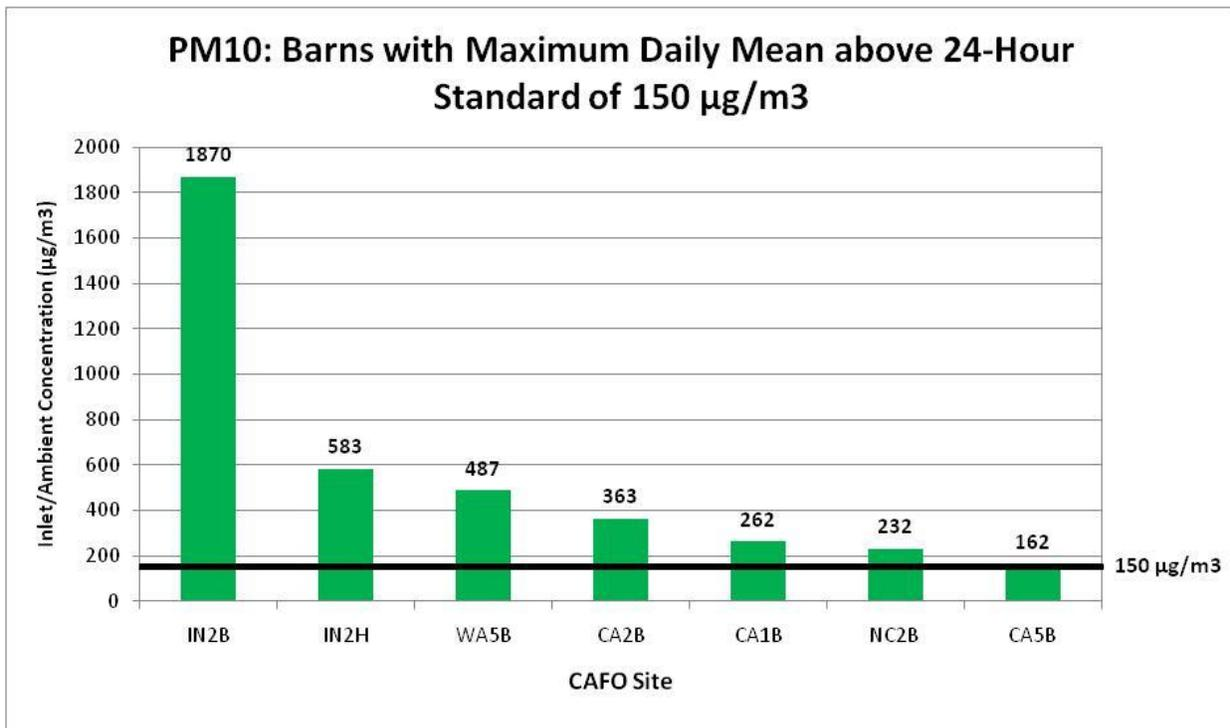
As shown above, inlet/ambient air at 7 of the 15 sites exceeded the PM<sub>10</sub> standard, and 4 sites had days with PM<sub>10</sub> levels more than double the standard. The Indiana egg layer site again had the highest readings. Air entering the IN2B facility reached 1,870 µg/m<sup>3</sup> on its worst day – more than *12 times* EPA’s 24-hour limit. In addition, all 7 of these sites exceeded the PM<sub>10</sub> standard on more than one sampling day during the study.
